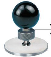
3. Place the metal shim between panel and control gauge base part. The hole is in order if you cannot push the gauge down to the round metal stop.
