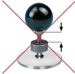
2. You can push the gauge down to the round metal stop with the metal shim in place. Fault: Drilling hole not deep enough. Drill bit worn out.
